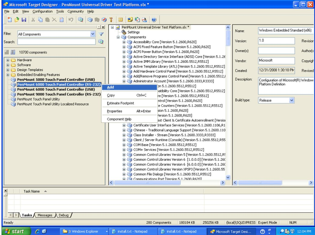
8. Run [ Configuration ] > [ Check Dependencies (F5) ] to add the components that the PenMount device depends on.
