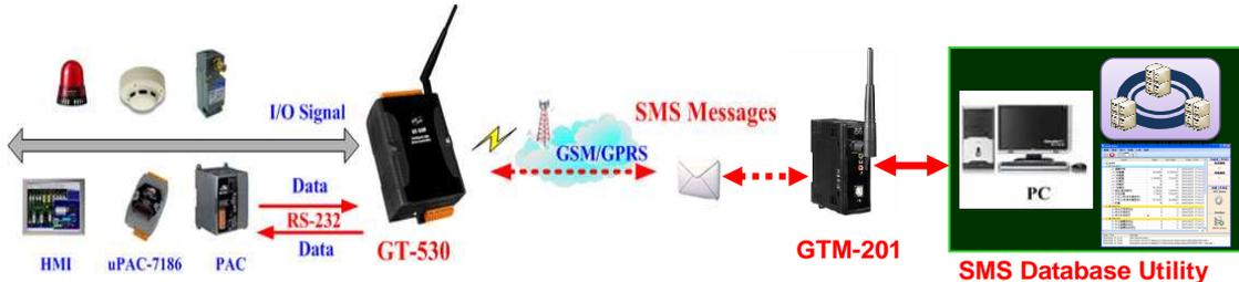
Before performing software installation, please configure GT-530/ GTM-201 hardware and set up the system (Figure above shows a possible system configuration. For more detail information, please refer to GT-530 User Manual.) Please be aware, The SMS Database System requires the .NET framework version 2.0 to be installed on the target computer. Please follow the link below to get the framework package directly from Microsoft, if required.
