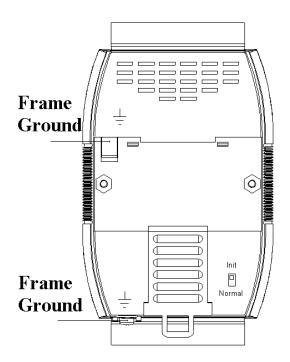
New DIN rail models are available that can easily be connected to the earth ground. Each are made of stainless steel, which is stronger than those made of aluminum. There is a screw at one end and a ring terminal is included as shown in the figure below. Refer to Section 1.13.1 for more information about the new DIN rail models.
