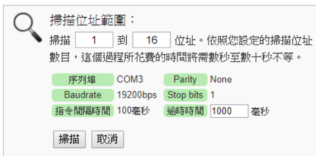
图7-4: 电测模块扫描范围设定
