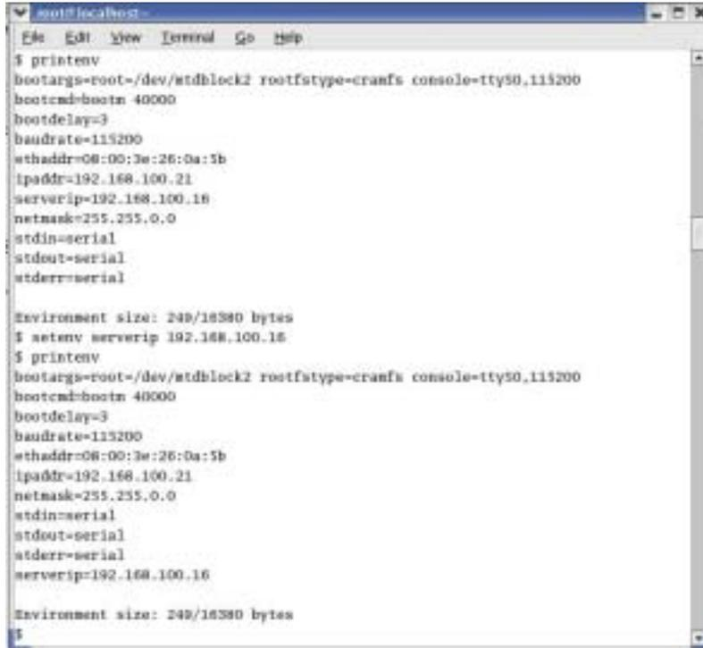
A terminal window titled 'root@localhost' showing the execution of 'printenv' and 'setenv' commands. The 'printenv' command displays various U-Boot environment variables such as bootargs, bootcmd, bootdelay, baudrate, ethaddr, ipaddr, serverip, netmask, stdin, stdout, and stderr. The 'setenv serverip 192.168.100.16' command is used to update the serverip variable, and a subsequent 'printenv' command shows the updated value.
