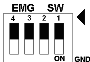
Fig. 1-14 EMG SW setting for user controlled signals.
