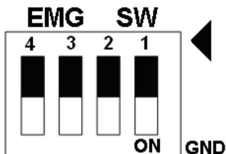
Fig. 1-14 EMG SW setting for user controlled signals.
