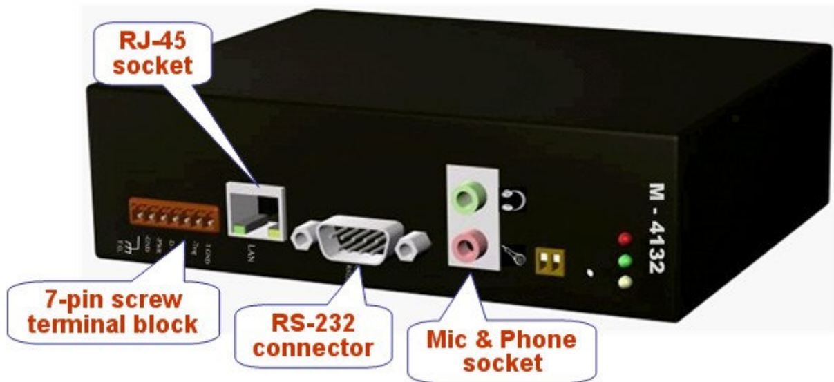
Figure 3: Pin assignment of M-4132
