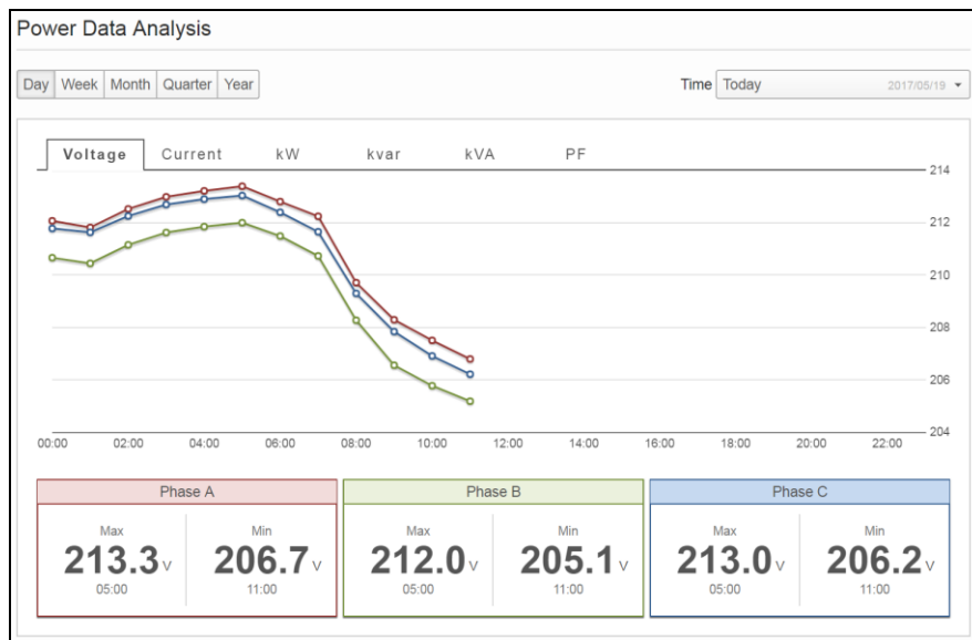
Figure 8-11 Historical Power Data - Power Data Analysis for Power Meter
