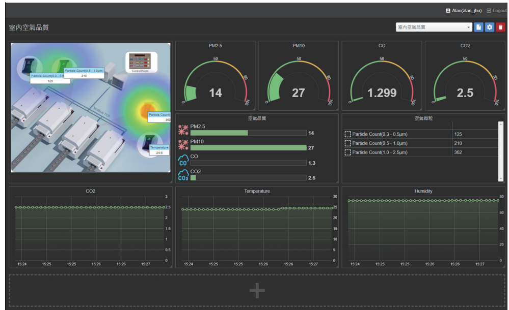
Example of Air quality monitoring (Using Line Chart, Gauge, Plot Bar, Value Table, Value Label Overlay widgets).
