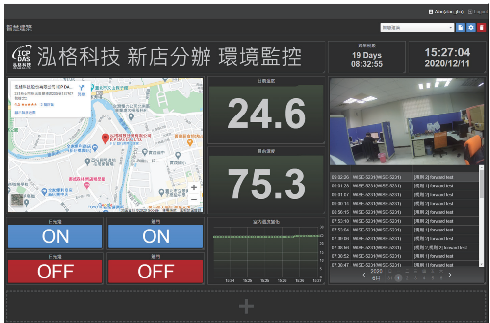
Example of Environmental monitoring (Using Line Chart, Value, Value Output, Map and Video Event List widgets).
