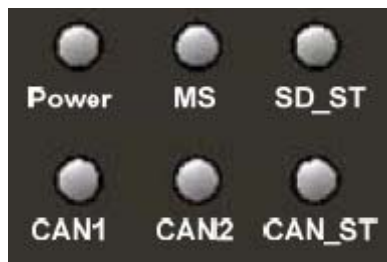
Figure 2-7 LED Assignment of CAN-Logger200
