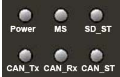
Figure 2-6 LED Assignment of CAN-Logger100
