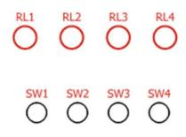
SW1 ~ SW4 are test push buttons that control Relay 1 ~ Relay 4 ON / OFF.
