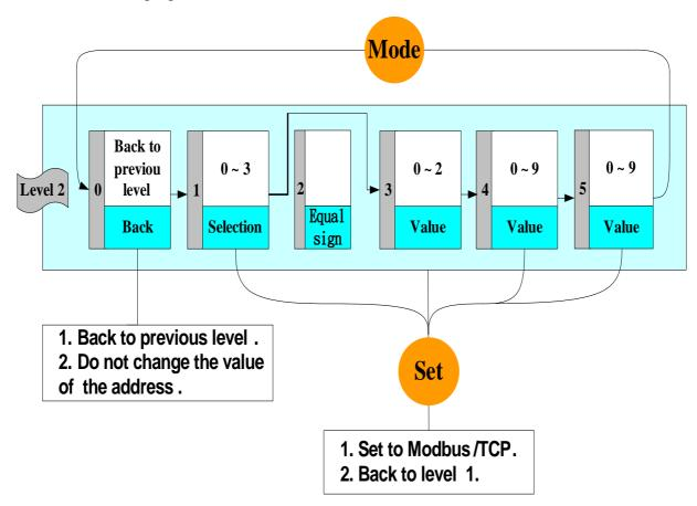
When entering the "**Set values procedure**", the LED shows the current value. The following example: show that the IP=192.168.255.1.
