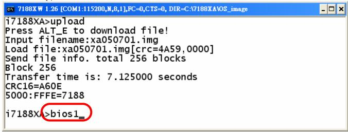
Step 8: It will take about 10 seconds to upgrade MiniOS7. After the update has finished, the system will automatically reboot. If this does not occur, the system must be rebooted manually.
