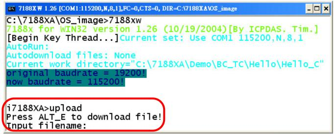
Step 5: Type the image filename (for example: xa050701.img) then press <ENTER>.
