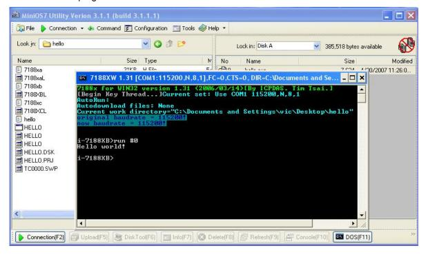
NOTE: The 7188xw window has to be closed and then the download operation (Step 5) could be done.
