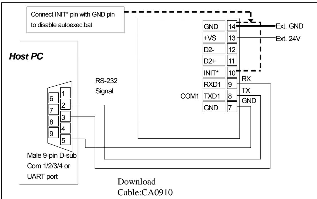
**Step 1:** Connect the module and Host PC with download-cable, CA0910/CA0910F. As shown in the above diagram.
