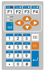
step 3, press '.' Key continusly until the red led on 'F4' turns on
