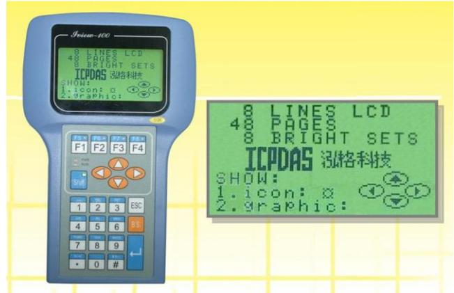
The iVIEW-100 series can be also used as a HMI device for our I-7188,  $\mu$ PAC-7186 and I-8000 series embedded controller. Since the basic hardware design of iVIEW-100 is similar to that of I-7188 series, all our available software can be used in iVIEW-100. User can design iVIEW-100 application with C Language. We will provide iVIEW-100E with a 10/100 mega Ethernet port for internet.
