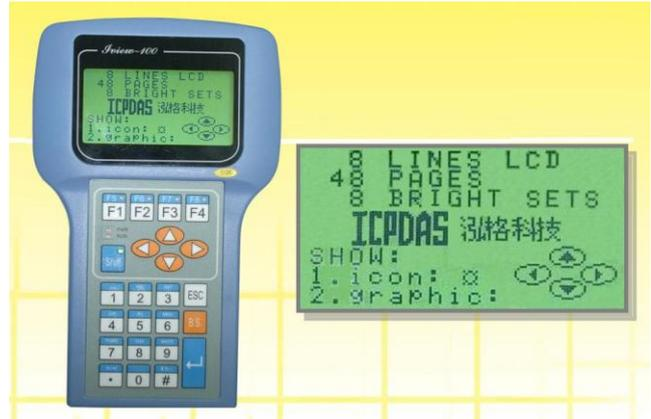
The iVIEW-100 series can be also used as a HMI device for our I-7188, μPAC-7186 and I-8000 series embedded controller. Since the basic hardware design of iVIEW-100 is similar to that of I-7188 series, all our available software can be used in iVIEW-100. User can design iVIEW-100 application with C Language. We will provide iVIEW-100E with a 10/100 mega Ethernet port for internet.
