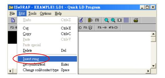
Or you could click the "F2 (Contact on the left)" tool button to insert a rung quickly.
