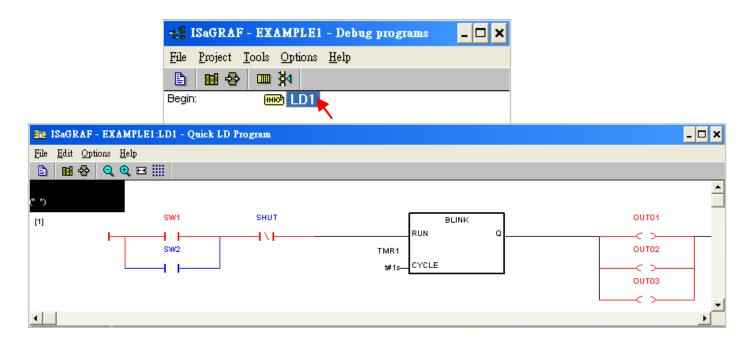
**Note:** The "SHUT" is a Normal Close switch that has been energized so its color is red. It is used in a concept of inverted phase, so the logic is "OFF", but not "ON".
