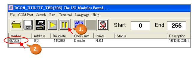
3. Now, you can set the Address, Baud rate and Checksum. After configuration, you **must** click "Setting" to save the settings.
