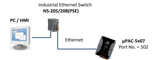
Before you can download an ISaGRAF application to the  $\mu$ PAC-5x07 PAC using the Ethernet port, you must first setup the Ethernet port to properly communicate with the host PC.
