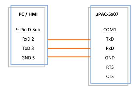
For the ISaGRAF Workbench RS-232 communications to operate properly, only the RXD, TXD, and the GND signals are used. If your PC is running a hardware device or software program that uses the RTS and CTS signals, then you will need to wire the RTS-CTS signals together.
