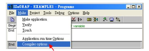
Make sure you have selected the following three necessary options in the "Compiler Options" window, and press "OK" button to complete the setting.
