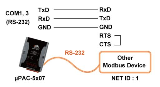
**Note:** COM3 ~ COM8 is optional from XW-Board (XW5xx), RS-232/RS-422/RS-485 expansion board.
