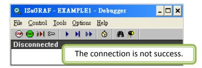
The most common causes of connection failure are the COM Port between each other is not plugged in or the settings of communication parameters are not correct. When this occurs, please follow the following steps to troubleshoot the problem:
