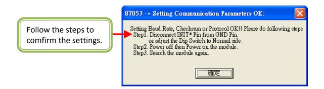
**Note:** Remember to remove the wire between INIT\* and GND, then restart the power if you use the I-7000 I/O module.
