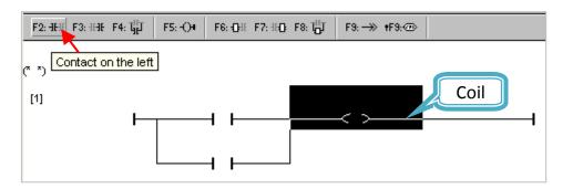
Then, click the "Contact" (as diagram below) and click the "Coil/contact type" tool button to set the attribute as "Normal Close".
