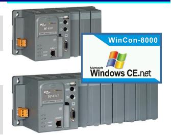
W-8337/8737 supports I-8K & I-87K I/O boards. There are more than 50 I/O boards available including DI, DO, AI, AO, Relay, Counter, frequency, Thermo-couple, RTD, Thermistor, Motion, ... Up to 224 local I/O channels can be used in slot 1 to slot 7. More I/O can be expanded by remote I-7000 (or I-87K) serial I/O modules or M-7000 series I/O via RS485 port.
