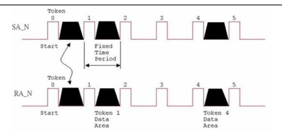
Figure 1.1 Token stream controlled by network manger, SA0
