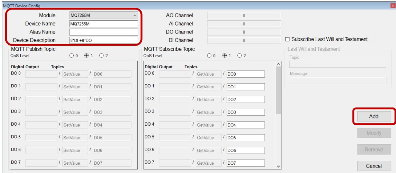
Refer to the MQ-7200M series user manual to check the Alias Name on MQ-7200M web interface.
