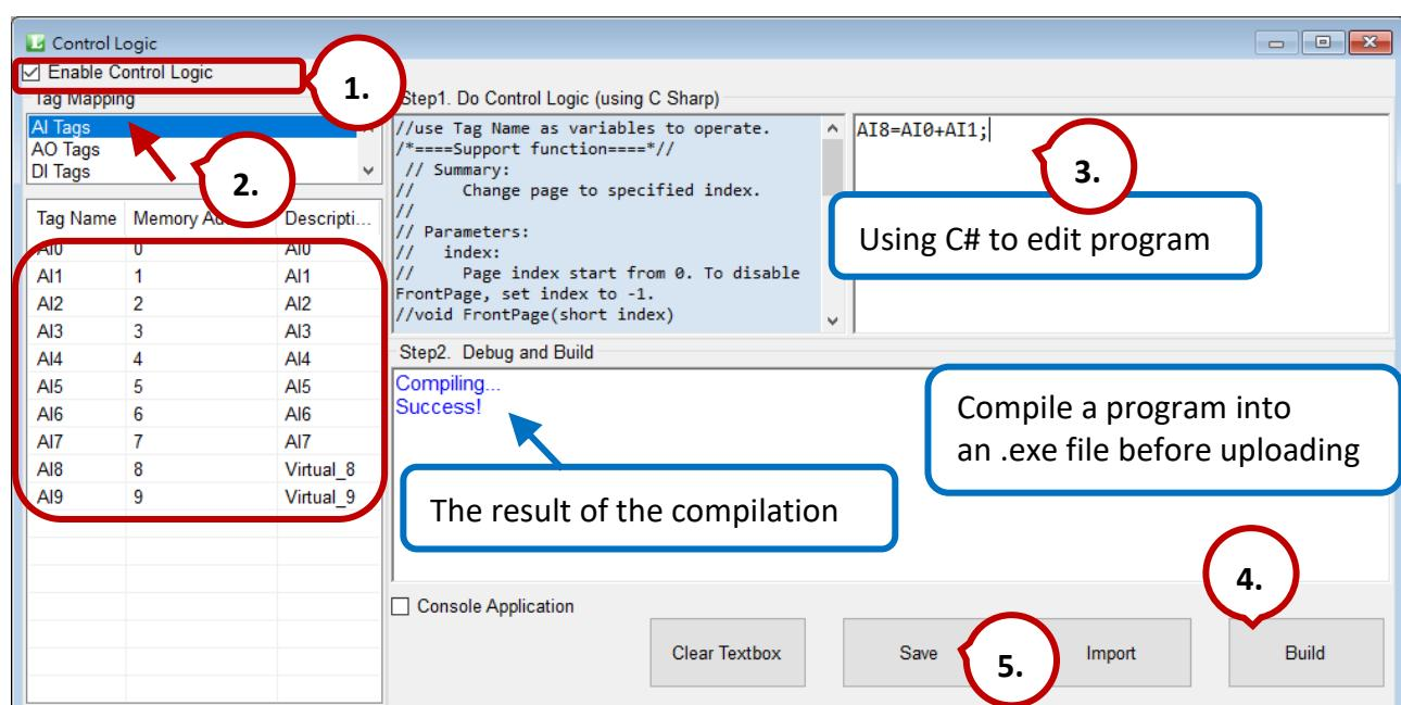
**Note:** After the compilation, a **ControlLogicRuntime.exe** file will be generated in the **Developer** folder of eLogger Developer.
