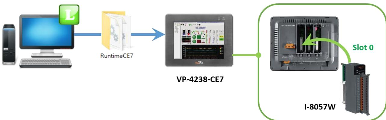
**Step2:** On PC, copy all files in the PAC Runtime folder (e.g., eLogger\_V201...\RuntimeCE7) and paste to **VP-4238-CE7** by using FTP or an USB drive.
