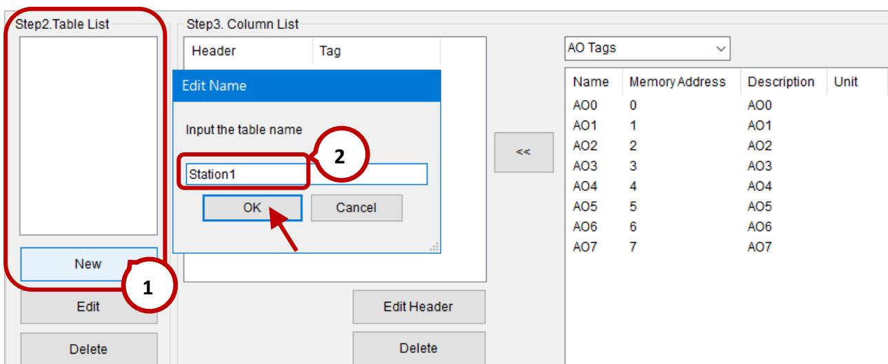
**Step4:** Click the table name and select the tag type, and then add the selected tag into the **Column List** one-by-one. Finally, click the **Set Setting** button to completing the setting.
