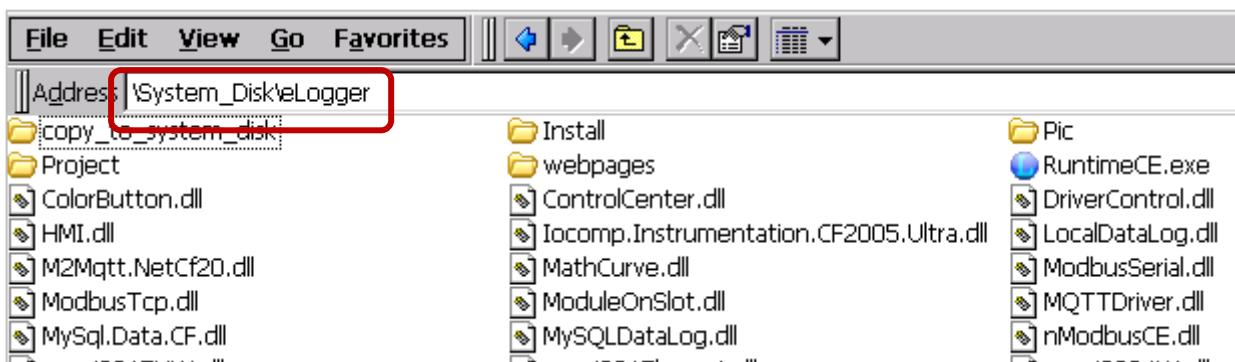
**Step3:** On PAC, copy dll files in the '\System\_Disk\ellogger\copy\_to\_system\_disk' folder and paste to the '\System\_Disk\icpdas\system' folder.
