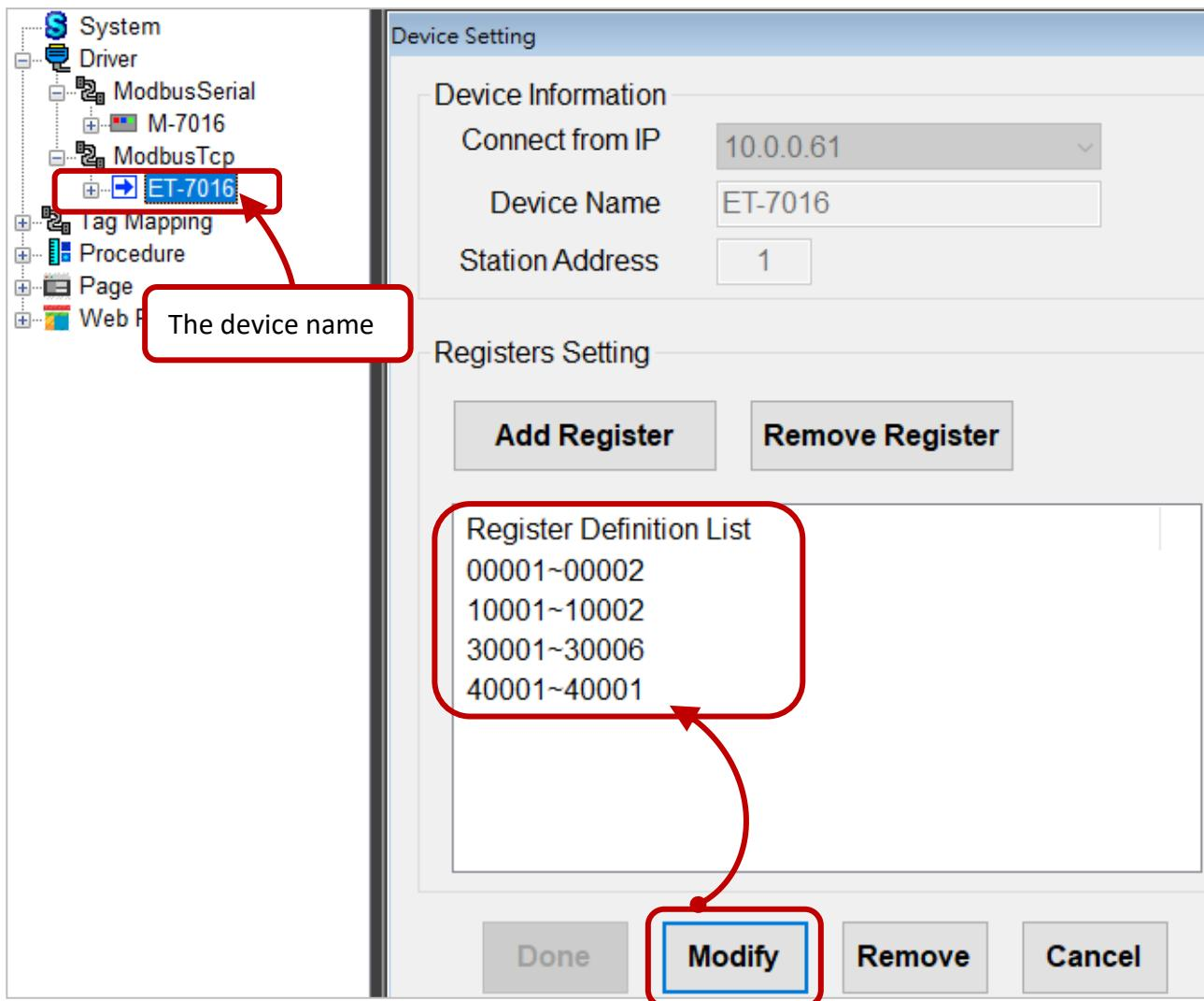
3. Expand the tree menu for the device name (ET-7016) to view all register name, and click the name to view the properties.
