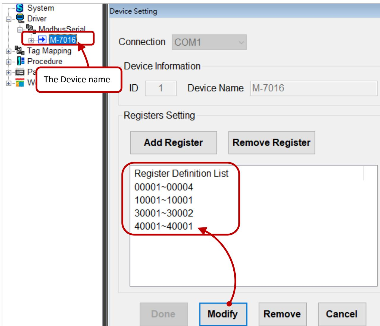
3. Expand the tree menu for the device name (M-7016) to view all register name, and click the name to view the properties.
