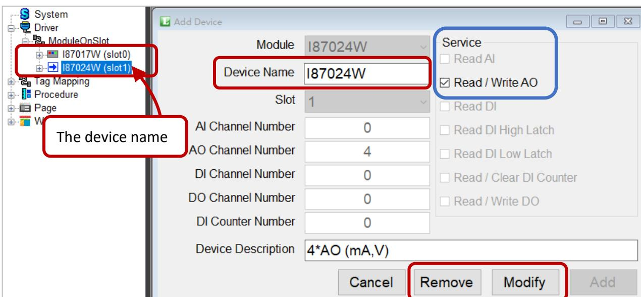
3. Expand the tree menu for the device name (I-87K) to view all register name, and click the name to view the properties.
