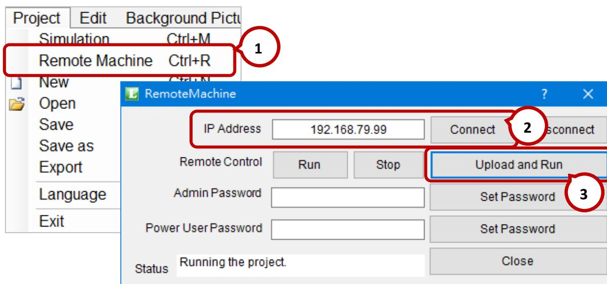
**Step4:** After the upload completes, the project will be automatically running.
