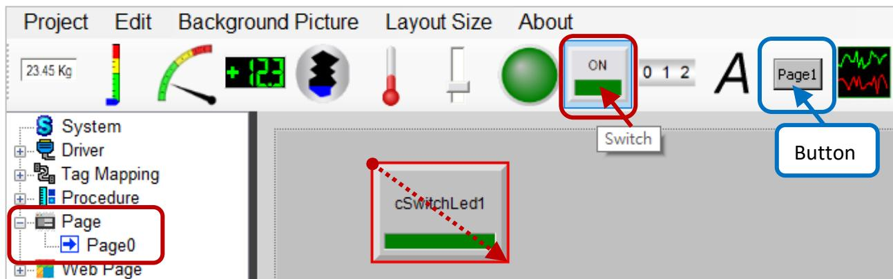
**Step2:** Click the object to display its property pane. Select **DO Tag** from **Tag Type**, select **D00** from **Tag Name**, and set **MouseControl** to **True** to allows set outputs with a mouse.
