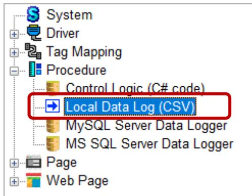
**Step2:** In the **Local Data Log Editor** window, check the **Enable Local Data Log** box to enable the function.
