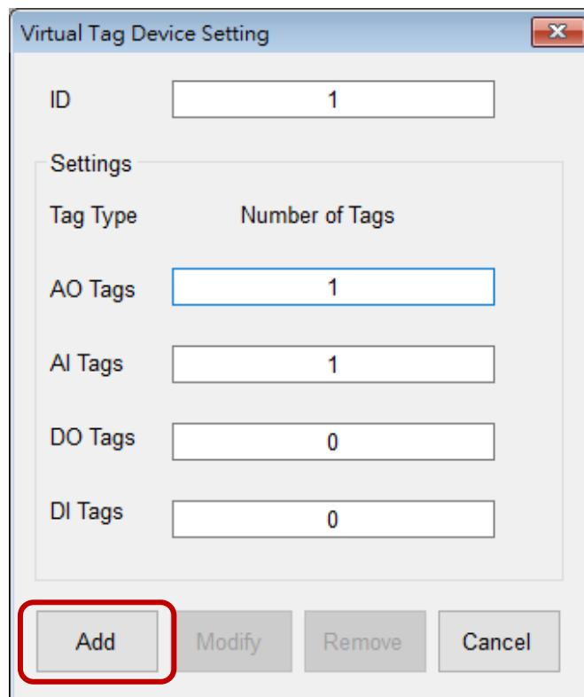
Users can check the added Virtual Tag Device in the **Driver** menu. In the **Tag Mapping** menu, the memory address for the added virtual tags will automatically be allocated. Click **New Tag** to add a tag and set the memory address and data type.
