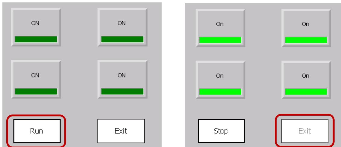
**Step6:** On PC (or smart phone, tablet), open the web browser and enter the IP address of the PAC, for example, <http://192.168.79.99/>, and then enter the username/password (defaults: admin/0000) to log into the web page. And then, you can remotely control the DO status of the module.
