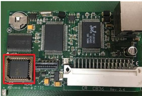
This type of IC can be plug out and replace easily, no need welding work.
