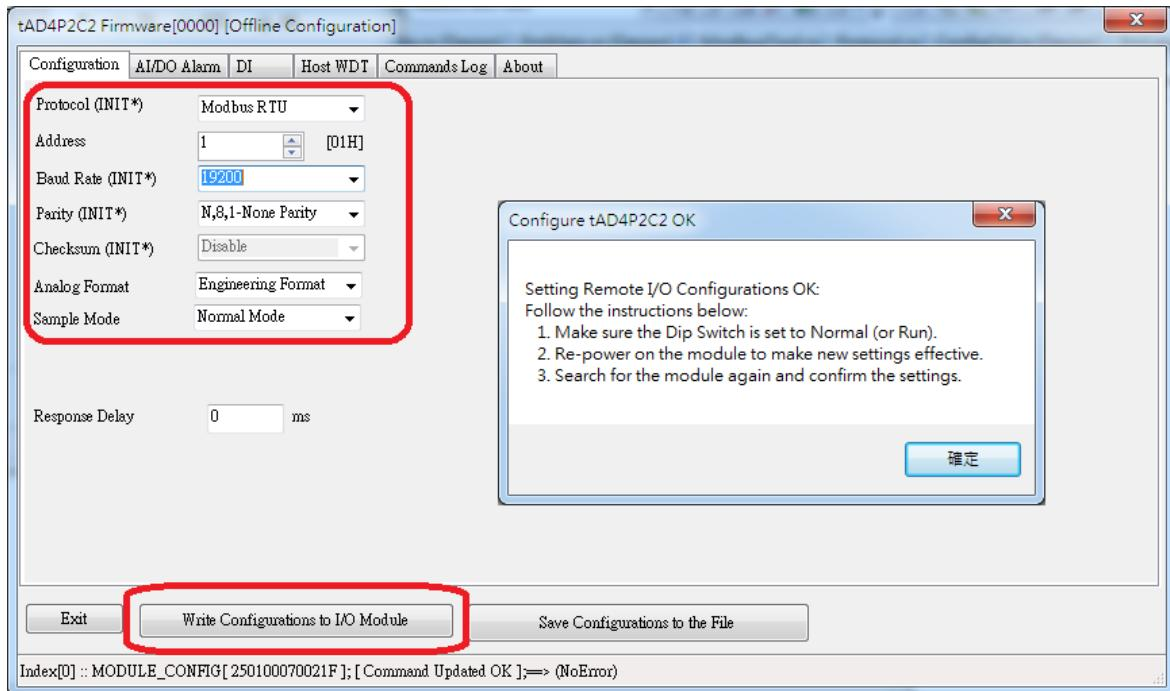
Note 1: Make sure to **power on module in INIT\* to GND** state the USB driver is correctly installed if use USB to RS-485 converter.
