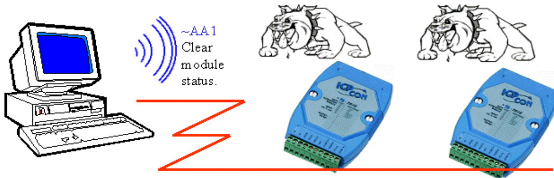
Figure 3. Host PC must use command ~AA0 to read the module status, and ~AA1 to clear the module status.
