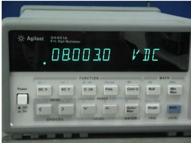
6 1/2 DIMM meter reads the real voltage : 8.003 V
