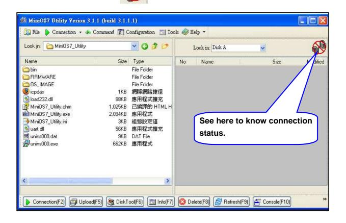
Step 4: Select the file to load from left side and click to load file into module or draw the file to the right side.
