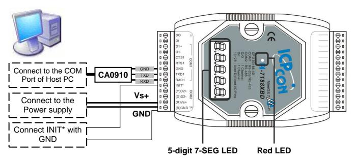
Step 3: After applying the power, the 5-digits of the 7-SEG LED will continuously show as follows.
