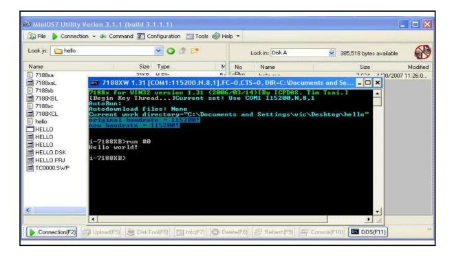
NOTE: The 7188xw window has to be closed and then the download operation (Step 4) could be done.
