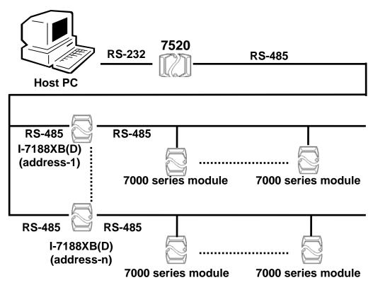
In this configuration, the 7000 series modules act as slave devices. The control programs are implemented in the Host PC. The operation steps are as follows:
