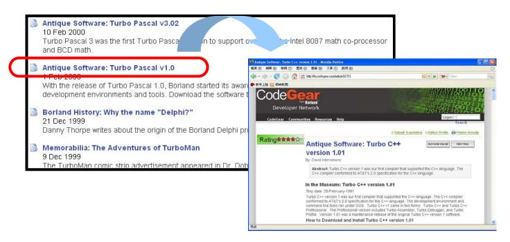
Step 3: Click on the link for **Turbo C++ version 1.01**, as shown below, to download the **tcpp101.zip** file. When requested, save the file to a safe location.
