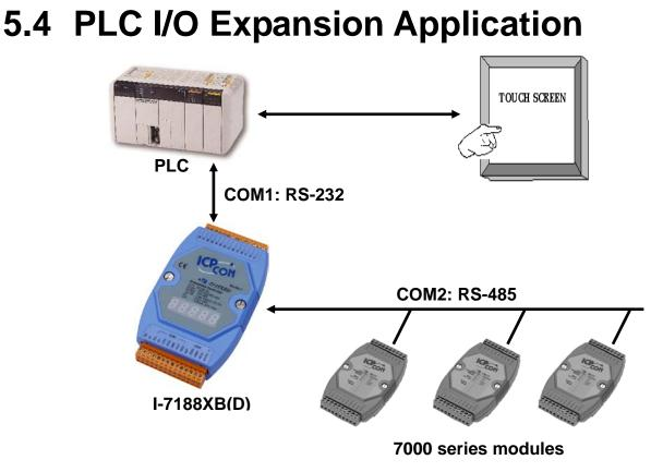
Most PLCs contain a Man Machine Interface that was originally designed for MMI applications. The I-7188XB(D) can use this interface to construct a bridge between a PLC and the 7000 series modules.
