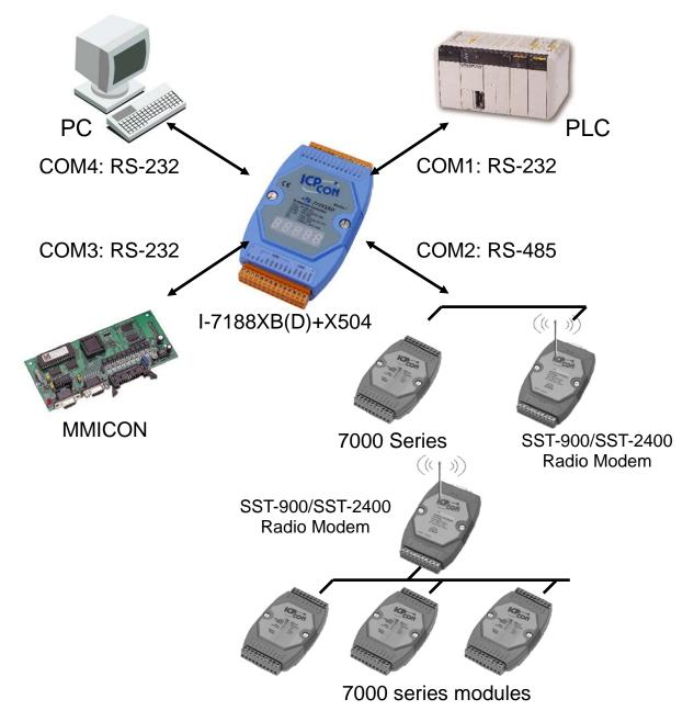
COM1: The PLC can access the I/O state of the 7000 series modules
