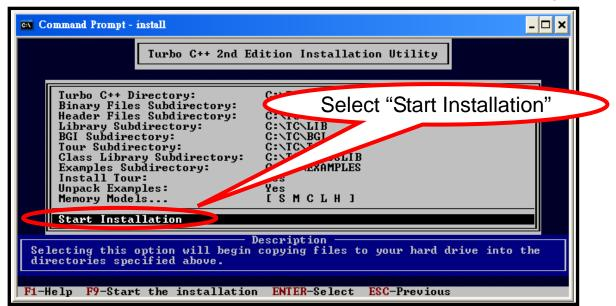
Step 5.6: At this point, the Turbo C++ version 1.01 compiler is installed in C:\TC, which is where the tcc.exe executable is also located.
