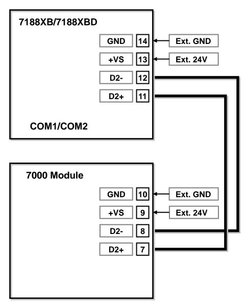
**Note:** The RS-485 interface can directly drive up to 256 I-7000 series modules without the need for a repeater.
