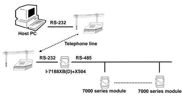
In this configuration, the control program is implemented series a local I-7188XB(D). The I-7188XB(D) will directly control the 7000 series modules based on these control arguments.
