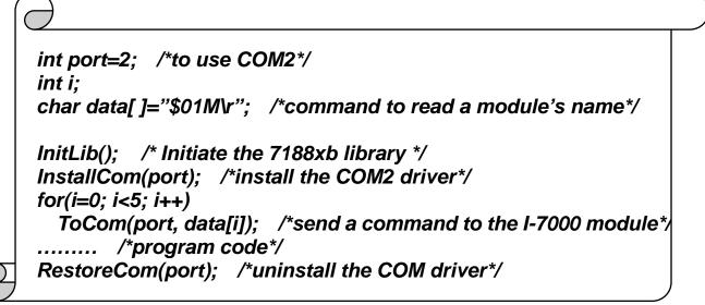
In addition to using the **ToCom()** function, the **SendCmdTo7000()** function can also be used to send commands to an I-7000 series module. The **ReceiveResponseFrom7000()** function can be used to receive the response from an I-7000 series module.
