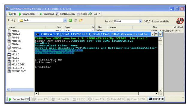
NOTE: The 7188xw window has to be closed and then the download operation (Step 4) could be done.
