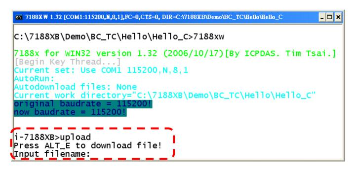
Step 5: Type the image filename (for example: xb050701.img) then press <**ENTER**>.
