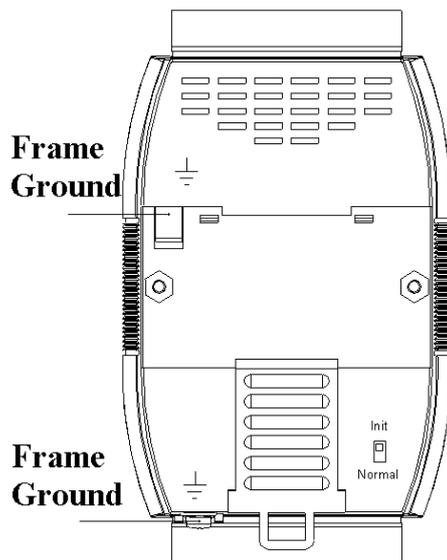
New DIN-Rail models are available that can easily be connected to the earth ground. Each rail is made of stainless steel, which is stronger than those made of aluminum. There is a screw at one end and a ring terminal is included, as shown in the figure below.
