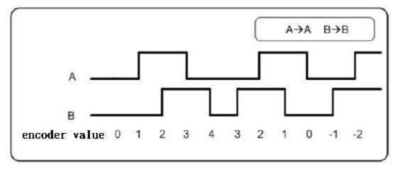
When InA0 is used as the A signal and InB0 is used as the B signal, the counter will be increased by one when the InA0 phase leads by 90 degrees to InB0 and the counter will be decreased by one when the InA0 phase lags by 90 degrees to InB0.
