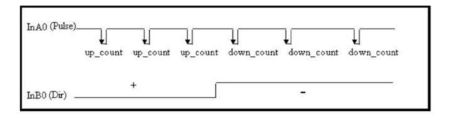
The InB0 is used for direction counting. When InB0 is high, the counter will be increased by one for every falling edge of InA0. When InB0 is low, the counter will be decreased by one for every falling edge of InA0.
