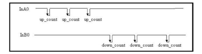
When InA0 is used as an up counting clock and InB0 is used as a down counting clock, the counter will be increased by one for every falling edge of InA0 and decreased by one for every falling edge of InB0.
