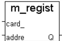
**Note:** If using "I\_8091A" rather than "I\_8091" on the I/O connection window, user don't need to call "m\_regist" & "m\_s\_nc", they are ignored. The card\_NO of "I-8091A" is equal to its slot No. I-8xx7: 0 ~ 7. W-8xx7: 1 ~ 7.
