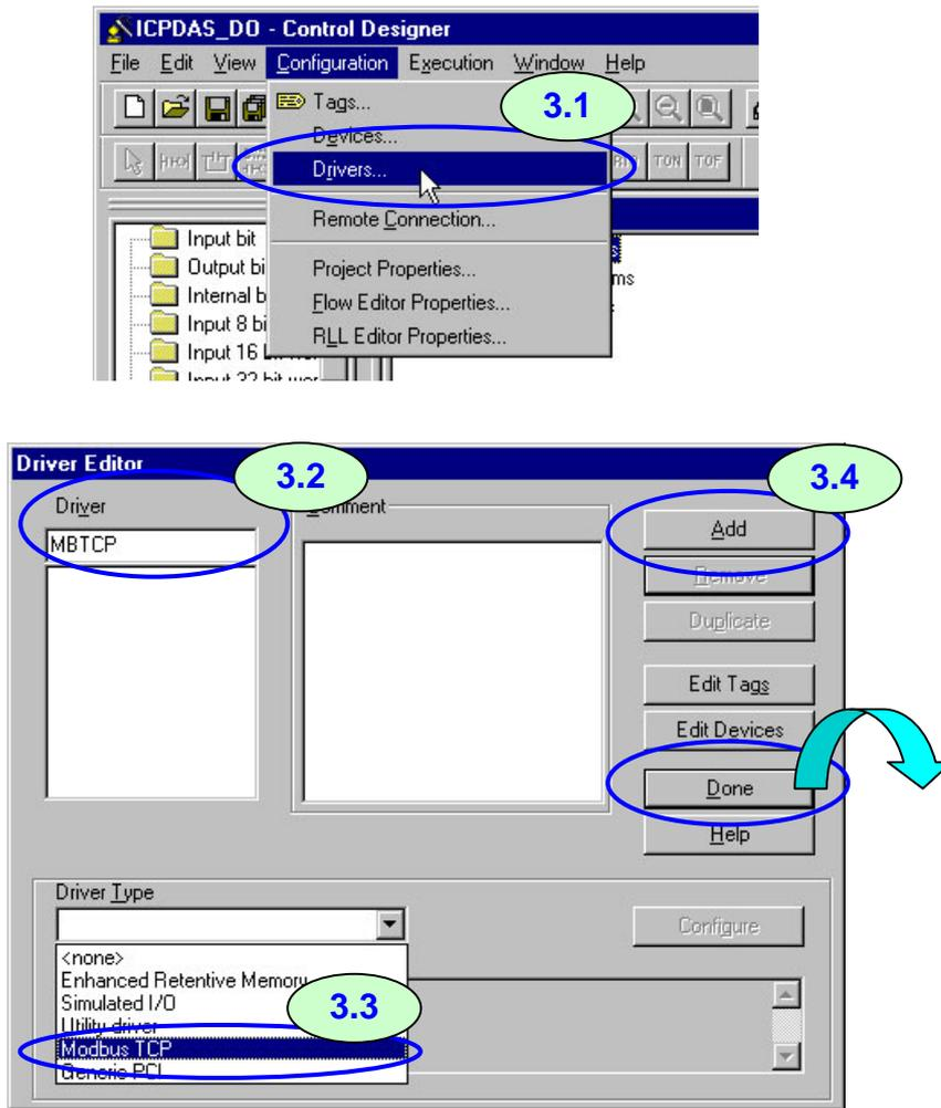
Step 4. Add all DOs as a Modbus/TCP station device. For example, named as **DO\_Station**.
