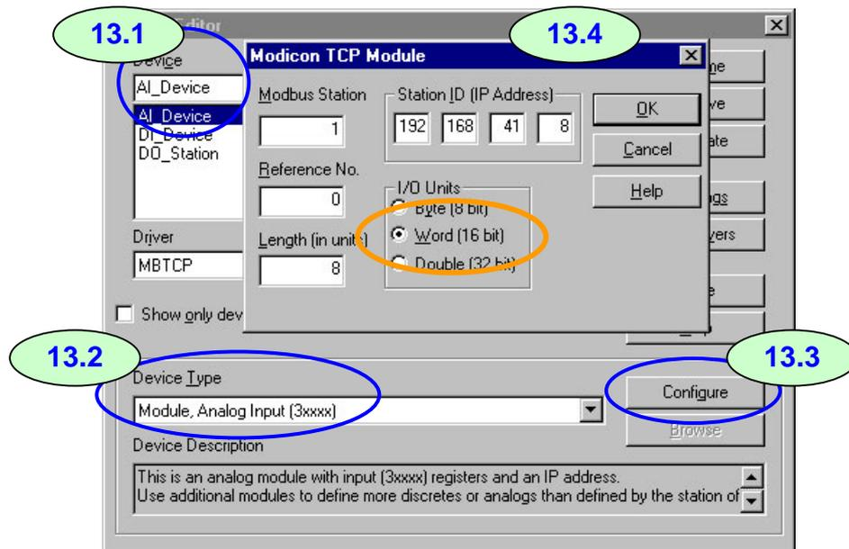
**Note:** every analog (AI and AO) register occupy 2 bytes, the I/O Unit must set to Word (16 Bits).
