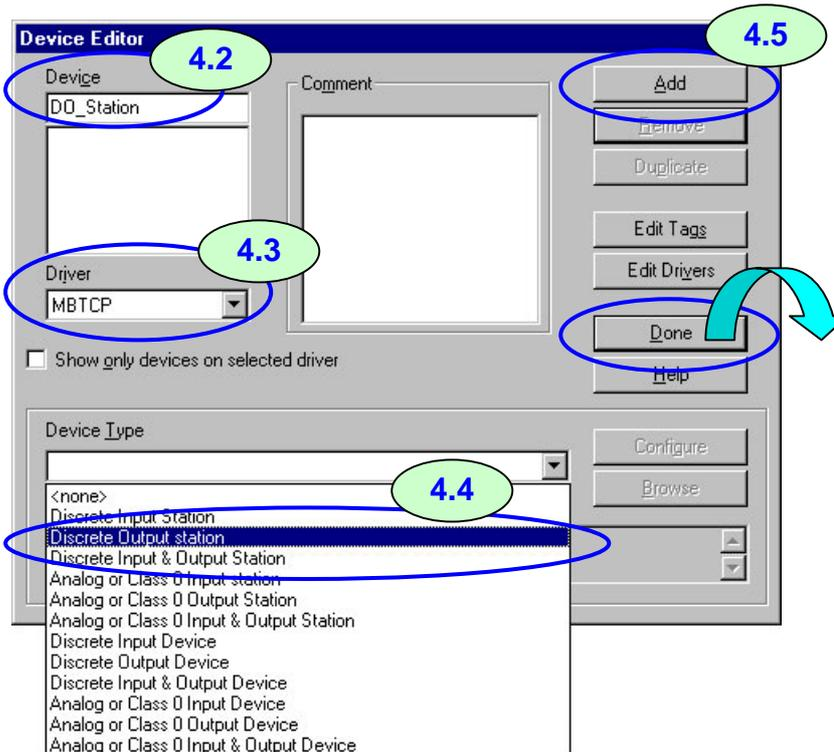
Step 5. Configure the Modbus/TCP station device.
