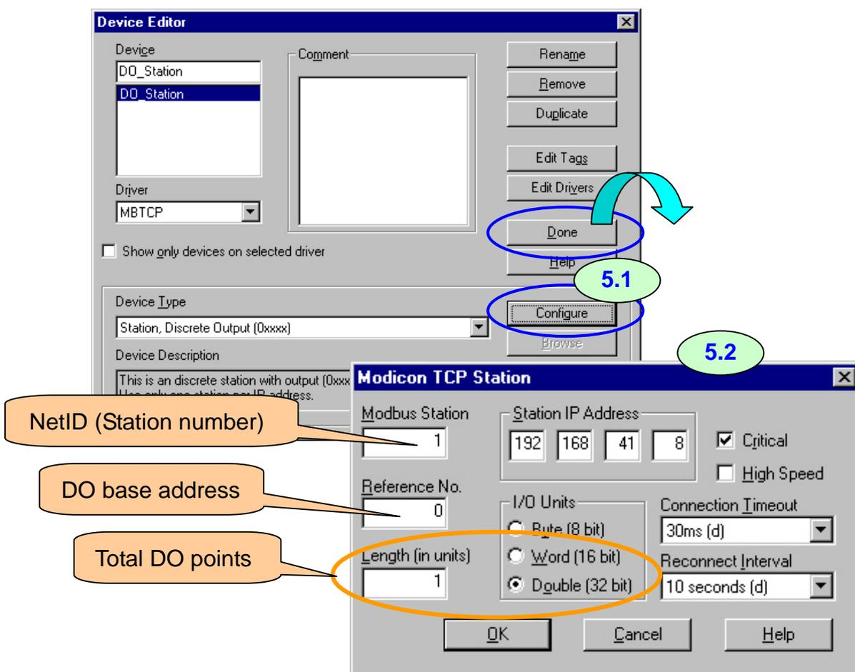
**Modbus Station:** also called NetID, for I-8000 controllers, you can find a dipswitch (at right side of controllers) to set the station number. After changing the station number, you must reboot the I-8000 controller.
