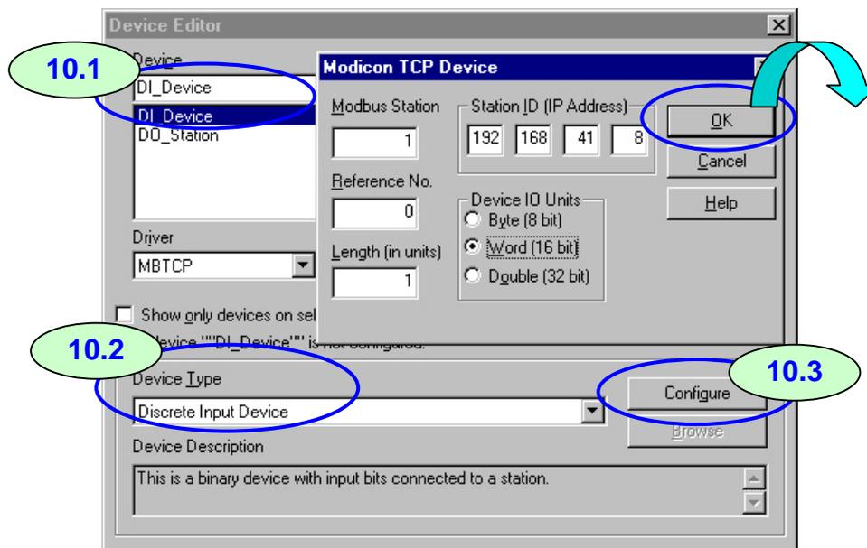
**Note:** You can mix different device type modules in one I-8000 controller. When you add the I-8000 controller to VLC, the first device type should be **Station**, and others should be **Devices**. That's why in step 5, the Device type I chose is Station, and here, I set it as Device.
