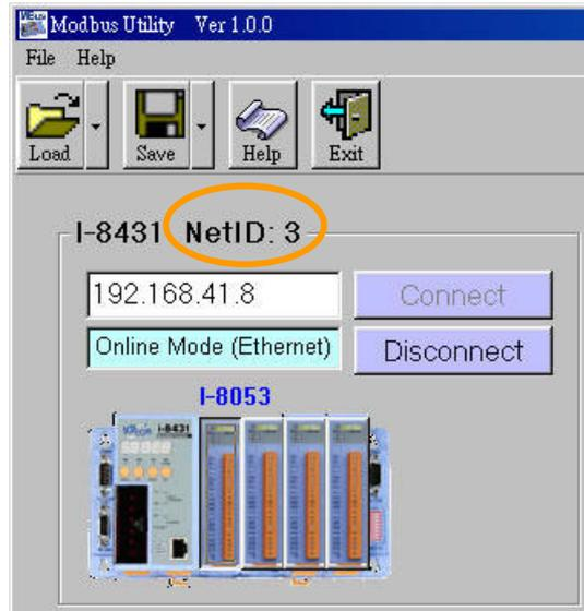
**Reference No:** you could plug several DO modules in one I-8000 controller. These addresses of points are continually. For getting best performance, you better group all DO modules, and only add one DO Modbus station or Modbus device to one VLC project. That VLC Modbus/TCP driver can set all DOs with one execution action.
