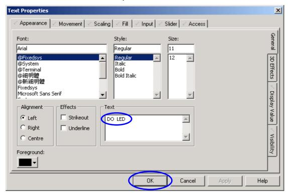
**Step27:** Follow the "Setp25" and "Step26" as a model, build three another Text Objects and put them in the appropriate place. The parameter setting of these Text objects are showed as following.
