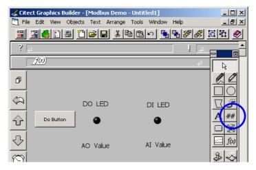
**Step29:**In the attribution-"Appearance", fill "Ao\_0" into the numeric expression field, and "Format" is "##.###". In the attribution-"Input", fill "####ENTER" into key sequence box, and fill "Ao\_0=arg1;" into command box.
