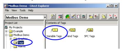
**Step16:** Input the Variable Tag Name, Select I/O Device Name, select appropriate data type, and correct address. All this parameters are shown as following table. When finishing the parameters setting of one tag, click "Add" to build the next tag.
