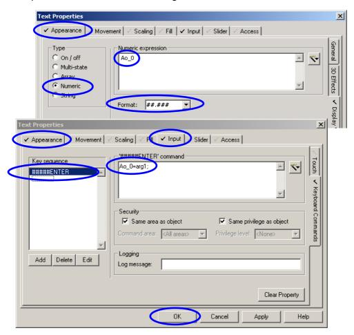
**Step30:** Follow the "Step29" as a model. Build a new number object, and set the "Appearance" attribution, but not to set the attribution-"Input". The setting parameters are as following.
