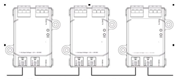
RS-485 and power input daisy chain using RJ-11 connectors
